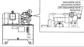
Adjust or set the discharge rate using the discharge rate adjusting screw; set the discharge rate using the length of the screw (dimension L) in the figure in the left as the reference. The relationship between dimension L and discharge rate Q is shown in the graphs below.
