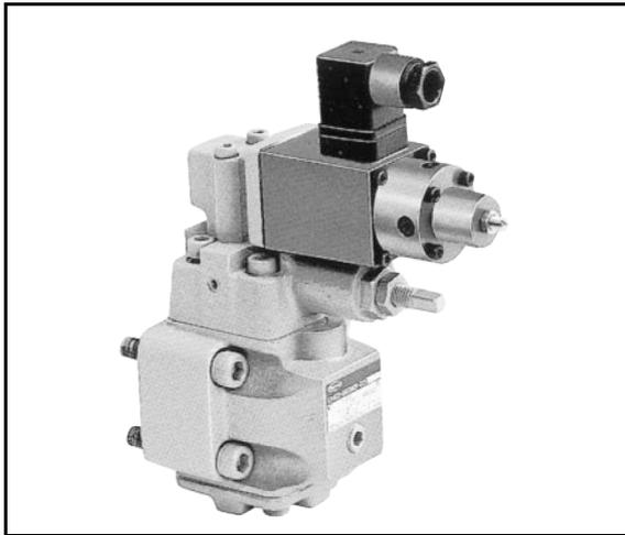
This current-controlled type pressure reducing valve controls the pressure by controlling the input current of the DC solenoid in the pilot section. This allows continuous and stepless remote control of the pressure.
